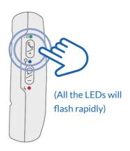
To turn on the device: press the top button for 1 second, all the LEDs will flash rapidly. The device can also be turned on automatically by charging via magnetic USB cable or putting it into the docking station.
